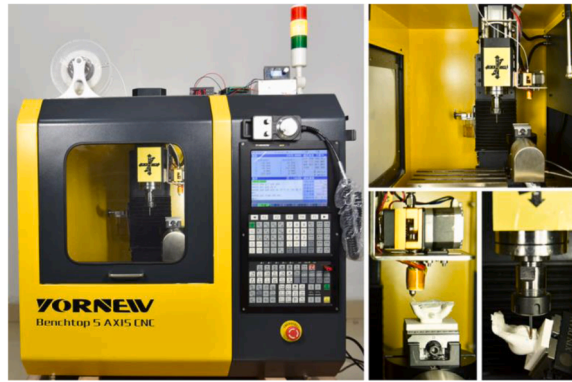
Fig. 39. The reinstalled machine tool and the additive-subtractive manufacturing process.
