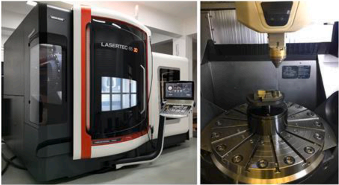
Fig. 1. The DMG LASERTEC 65 3D Hybrid integrates an additive manufacturing system in the conventional CNC machine center.
