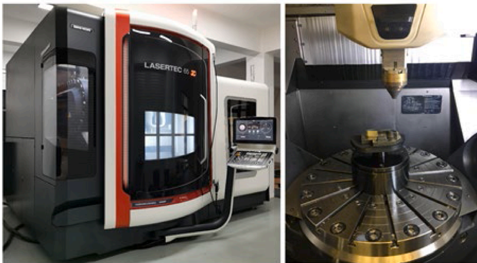
Fig. 1. The DMG LASERTEC 65 3D with a multi-axis additive manufacturing system.
